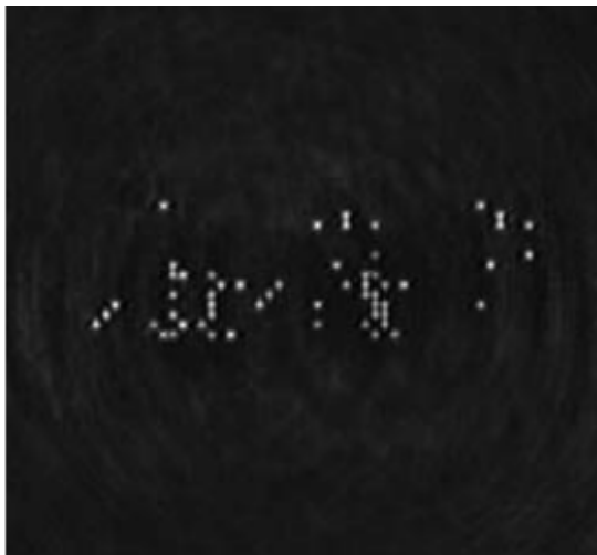
Fig. 5. Holographic memory pattern (700 × 700 pixels) including a two-bit multiplier circuit.
